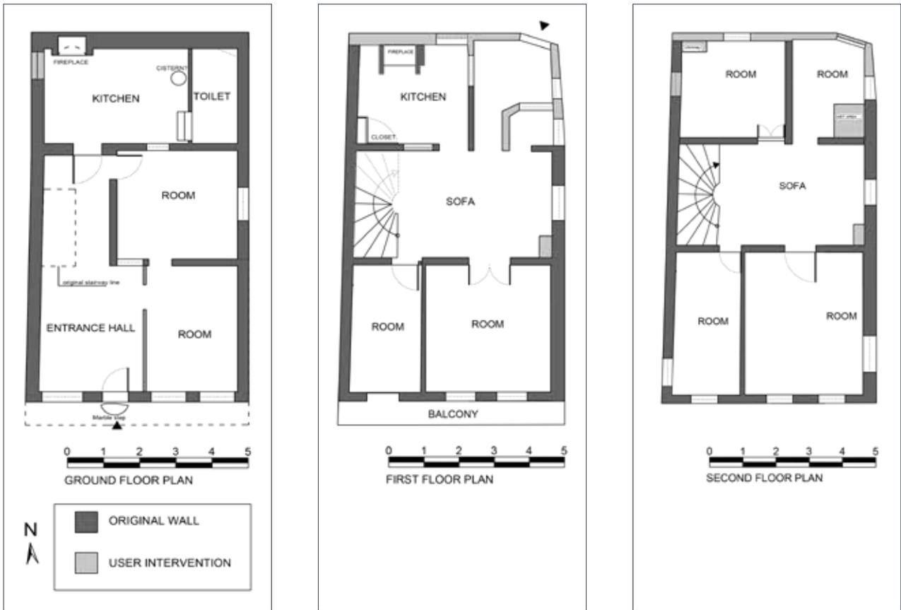
ground floor is a series of timber beams carrying planks, indicating a balcony; the south-western room on the first floor has a doorway opening onto this balcony (Fig. 3). A balcony along the entire façade is a feature rarely attested in traditional Turkish house architecture. The second floor projects out entirely.
